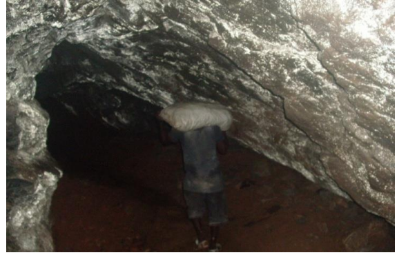
Fig. 7 A Miner Carrying Broken Material out of a Stope
