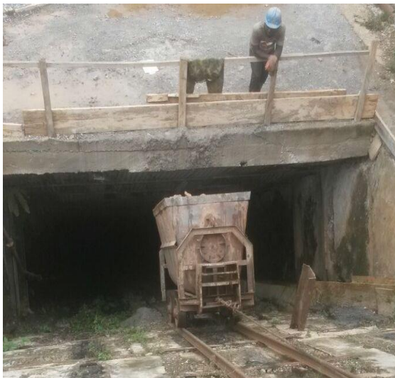
Fig. 9 Wagon and Winder Station in Semi-mechanised Operations
