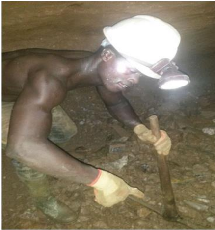
Fig. 5 Excavation of Materials using Pick
