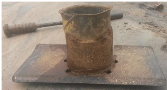
Fig. 2 Metallic Mortar and Pestle for Pounding Samples
